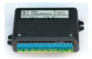
**Link Lift Watch provides communication** between a lift cabin and hotline service (first aid) via PSTN network. After pressing the alarm button on the control panel in the lift cabin the Link Lift Watch automatically dials up preprogrammed number (up to 6) and establishes connection with hotline service (first aid).
